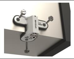
1<sup>st</sup>step - Attach the duct corner hanger to bottom corners of duct with self-drilling screws (Not provided by GPL). Three fixing screws required for one hanger. Please ensure the rubber pad should be available with all hangers because it prevents air leakage & vibrations. Above process to be done at floor level.
