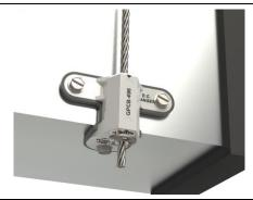
3<sup>rd</sup> step - After the fitting of wire with the hanger, we can hang the ductwork system with a suspension system. At least 100mm wire should reflect from bottom side of hanger as a tail to allow the future adjustment.
