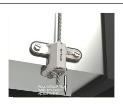
4<sup>th</sup> step - If need to re-adjust the placement, then pull the circlip of beam clamp to wire adjustment and release.
