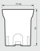
GP-04B: B-22 Candle Lampholder, 10mm entry thread with earth tag.
