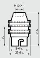
**GP-015**: B-15 Brass Lampholder, 10mm or ½" entry thread, with shade ring and earth tag.
